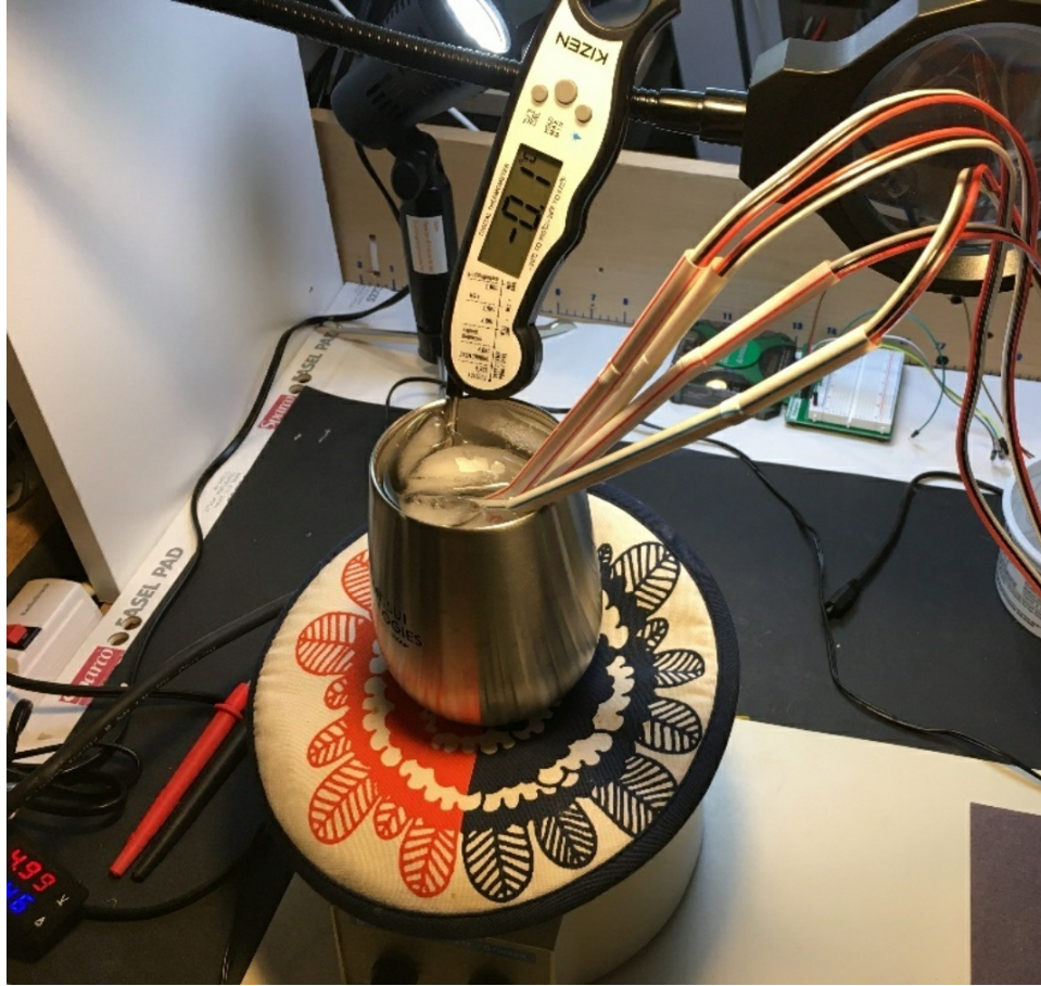
Figure 8.1 An ice bath with circulating water, ice, four sensors and the digital thermometer.
