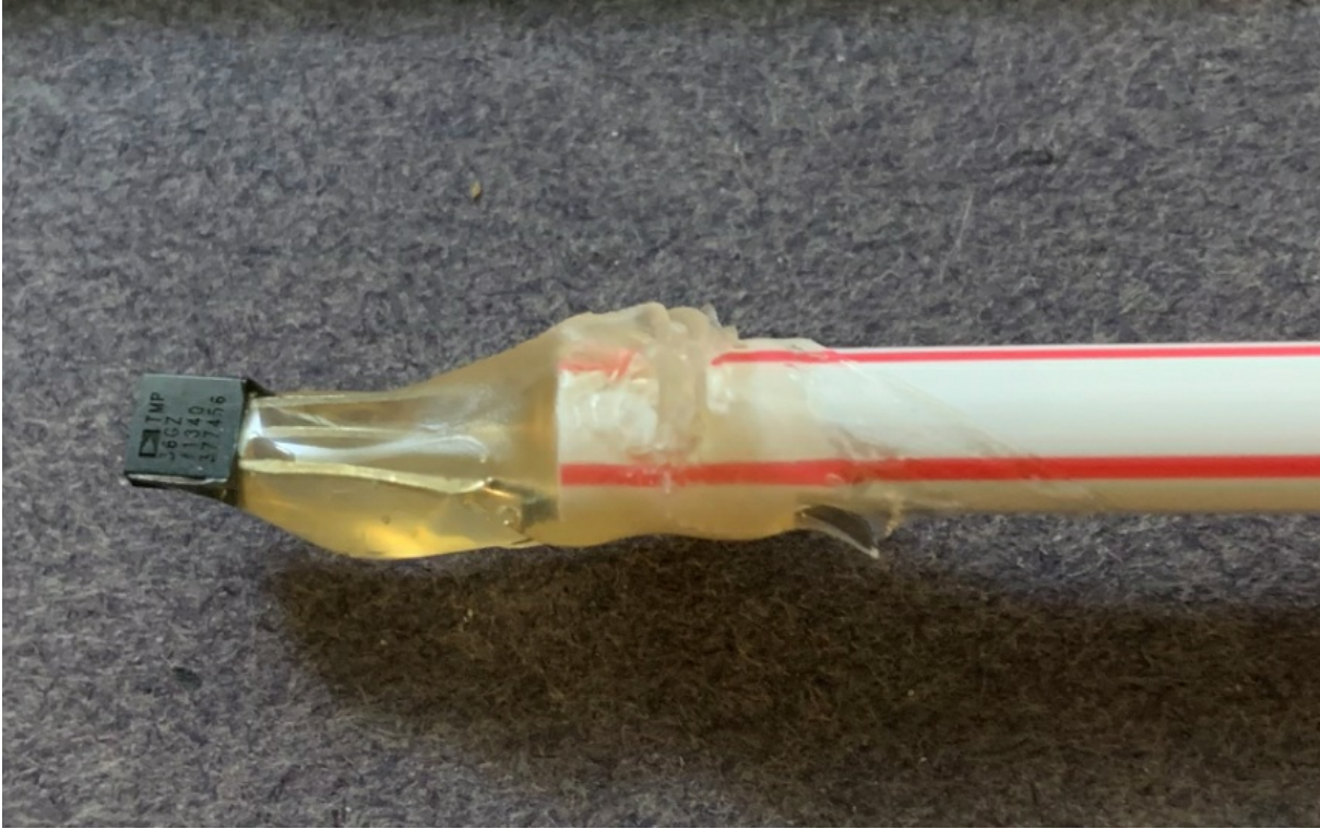
Figure 5.5 Close up of the TMP36 sensor with three wires soldered on the end and potted in hot glue then mounted inside a straw.
