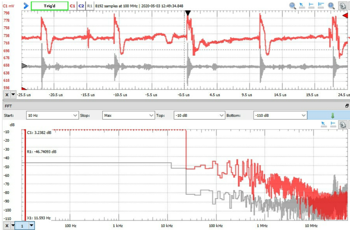
Figure 6.6 Measured noise with the TMP36 cable plugged in, in red, and the previous measurement of the dummy shorted cable, in grey. The voltage plots are on the same scale.
