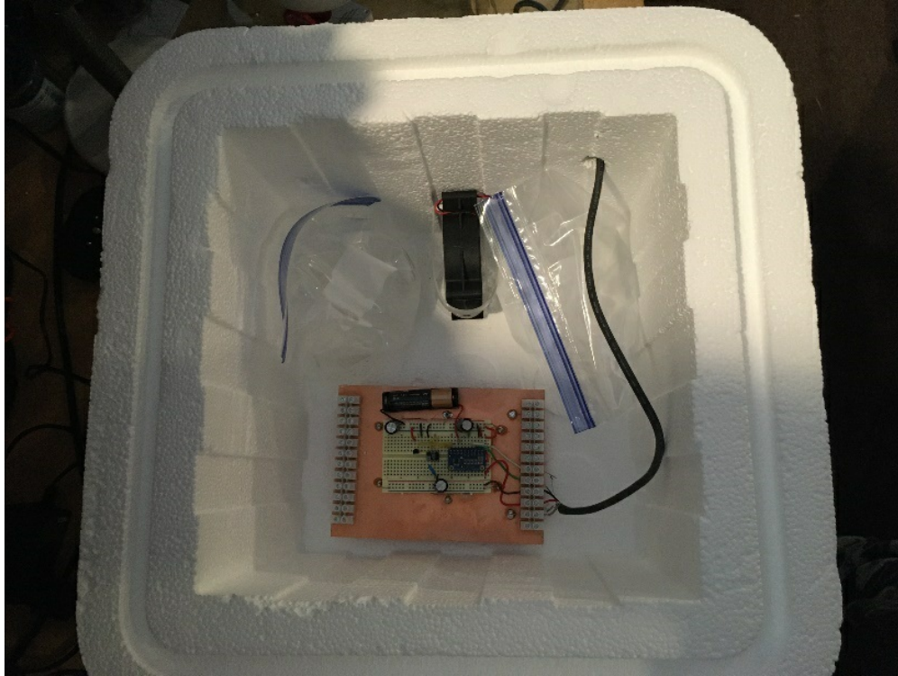
Figure 8.3 Inside the thick walled Styrofoam box with two bags of ice and a small circulating fan.
