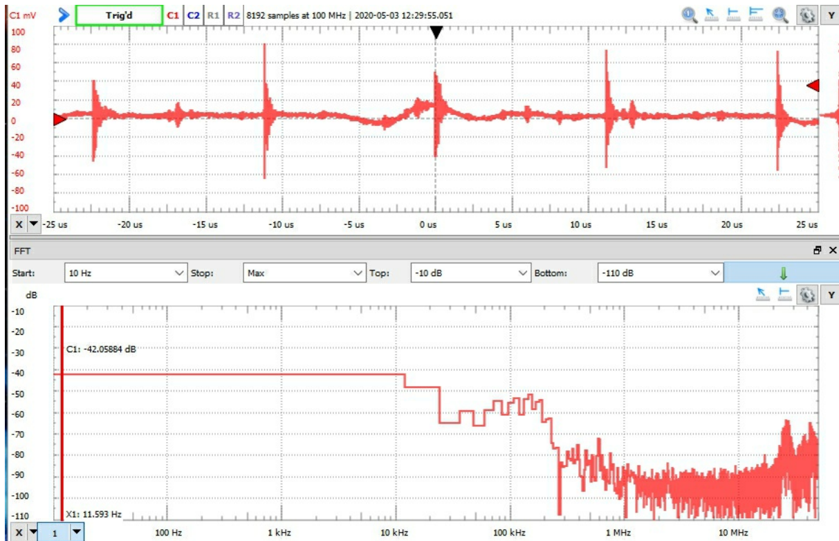
Figure 6.4 Measured noise pick up with the leads open, on a shorter time scale. Note the small peaks at about 25 MHz. This is the frequency of the ringing transients.
